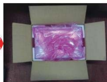
Then put anti-static bag into carton which has EPE cushion in it
